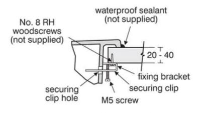
section through basin showing securing clip
