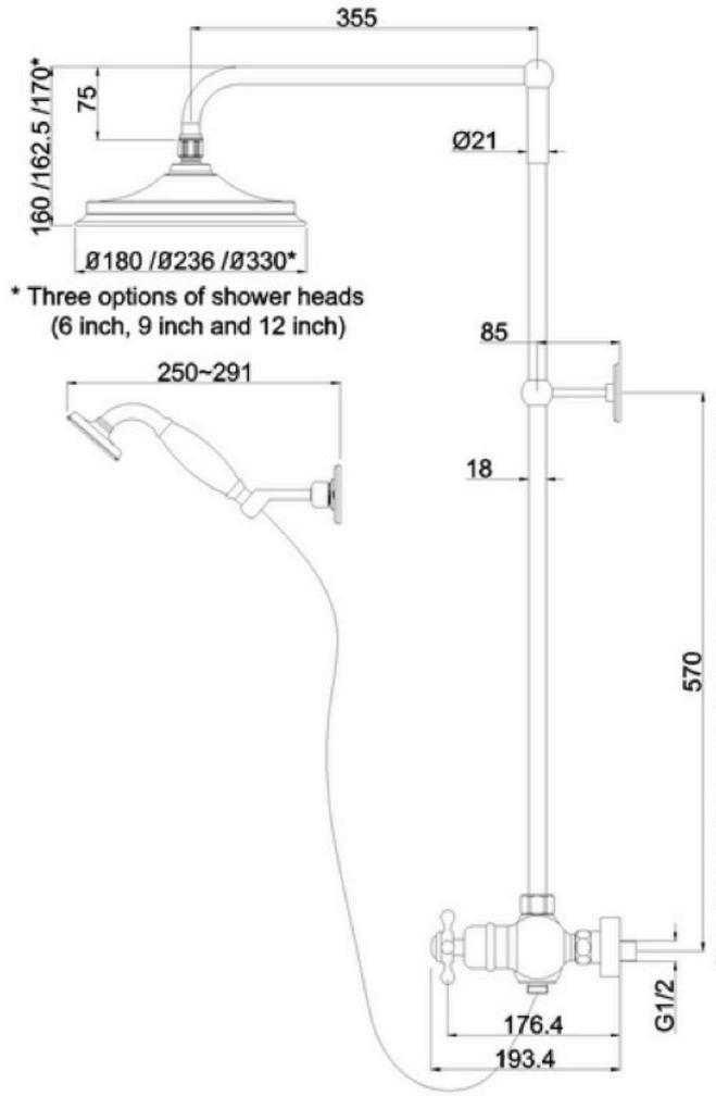
\*This dimension is recommended dimension without cutting the riser.
