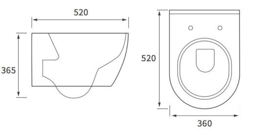
Coupling to soil stack: Horizontal
