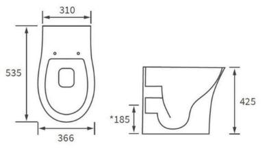
Coupling to soil stack: Straight out and straight down
